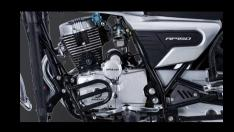
It adopts a 150CC single-cylinder fourstroke engine, which is naturally aircooled and starts with electric feet
