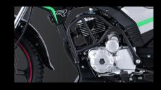
It adopts a 150CC single-cylinder fourstroke engine, which is naturally aircooled and starts with electric feet
